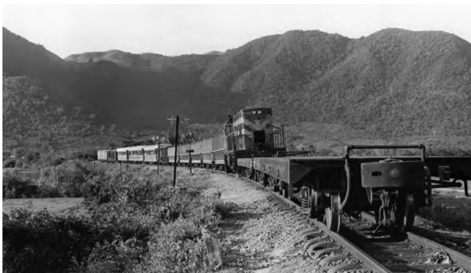
Flatcars on front of a train south of Phu Cat were intended to detonate mines placed on the tracks by the Viet Cong.
